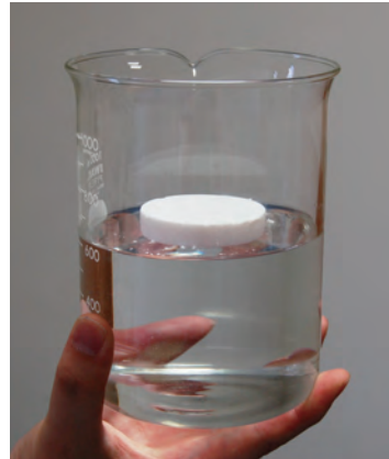
Ultra-low density porous aerogel
