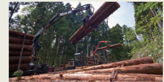
"Grapple crane trucks" are equipped with special cranes designed for use with logs, and they speed up loading work and help reduce timber transporting costs.
