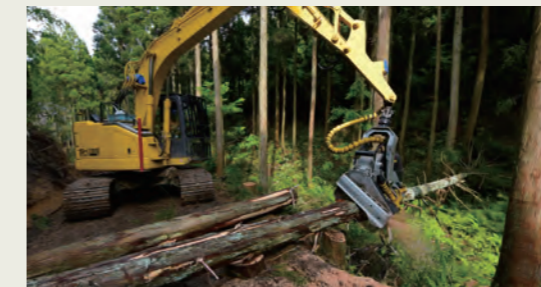
New "harvester" machines are able to carry out tree felling, pruning, and bucking, and timber gathering work, and are capable of carrying out such work roughly eight times more efficiently than conventional methods using chainsaws.
