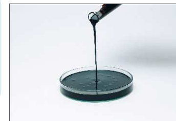
Black liquor (A biomass fuel made from resin content of wood chips, the raw material of pulp)
