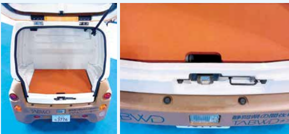
Vulcanized fiber used in the cargo bed of the Shizuoka Mokumaru vehicle
