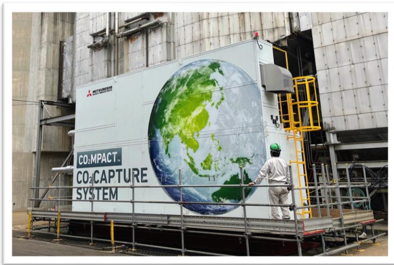
Compact CO 2 separation and recovery device (CO 2 MPACT™ Mobile, Mitsubishi Heavy Industries, Ltd.)
